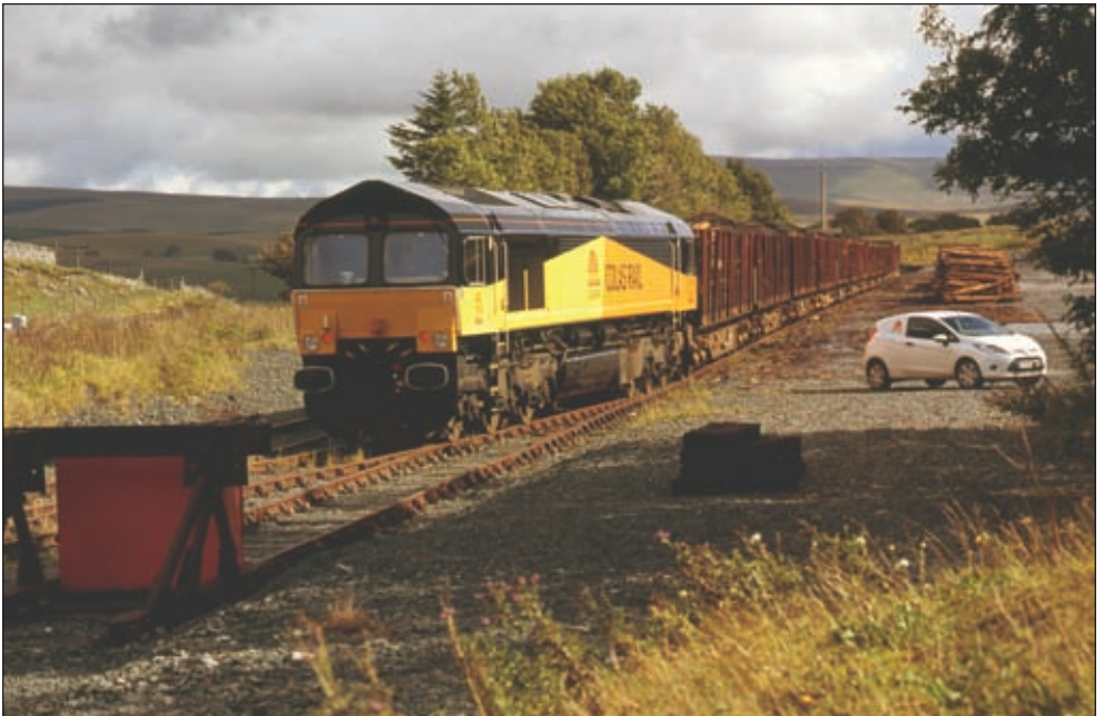
Above: The timber wagons are converted from old cargo vans, cut down and strengthened with stanchions to hold the logs in place. Below: 66841 worked the train on 20th September. Photos: Pete Shaw
