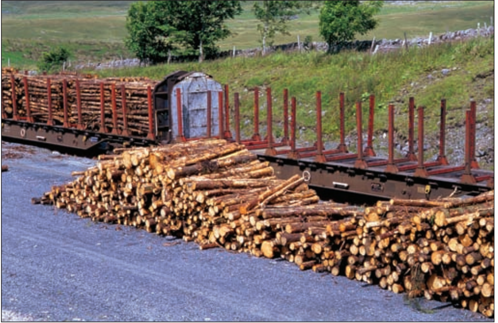
Above: The timber wagons are converted from old cargo vans, cut down and strengthened with stanchions to hold the logs in place. Below: 66841 worked the train on 20th September. Photos: Pete Shaw
