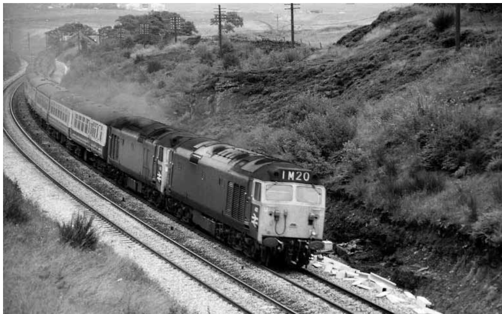
Above: Greenholme – In August 1971 1M20 10-00 Glasgow Central–Euston ‘Royal Scot’ descends Shap Bank at Greenholme with Two EE Type 4s in charge. Note the new concrete cable route troughing in the Up cess waiting to be installed for the modernised railway.
